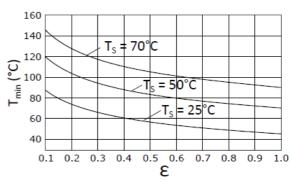
Graph showing the minimum measurable object temperature (Tmin), determined by surface emissivity ( $\epsilon$ ) and sensor temperature (TS).
